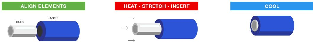
Haskel has developed a method for mitigating HEE that involves fitting a liner within the jacket of the high-pressure vessel. The liner has an outer diameter that is slightly larger than the jacket's inner diameter. The process involves three steps:
